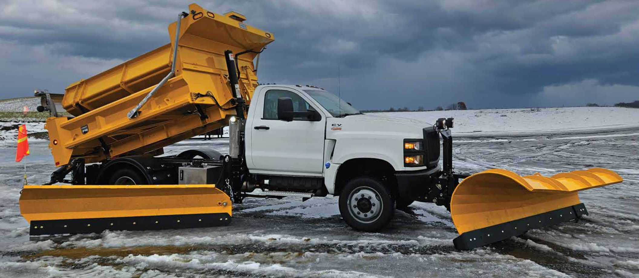
CV515 Everest turnkey snow removal truck, with side tilt dump body
