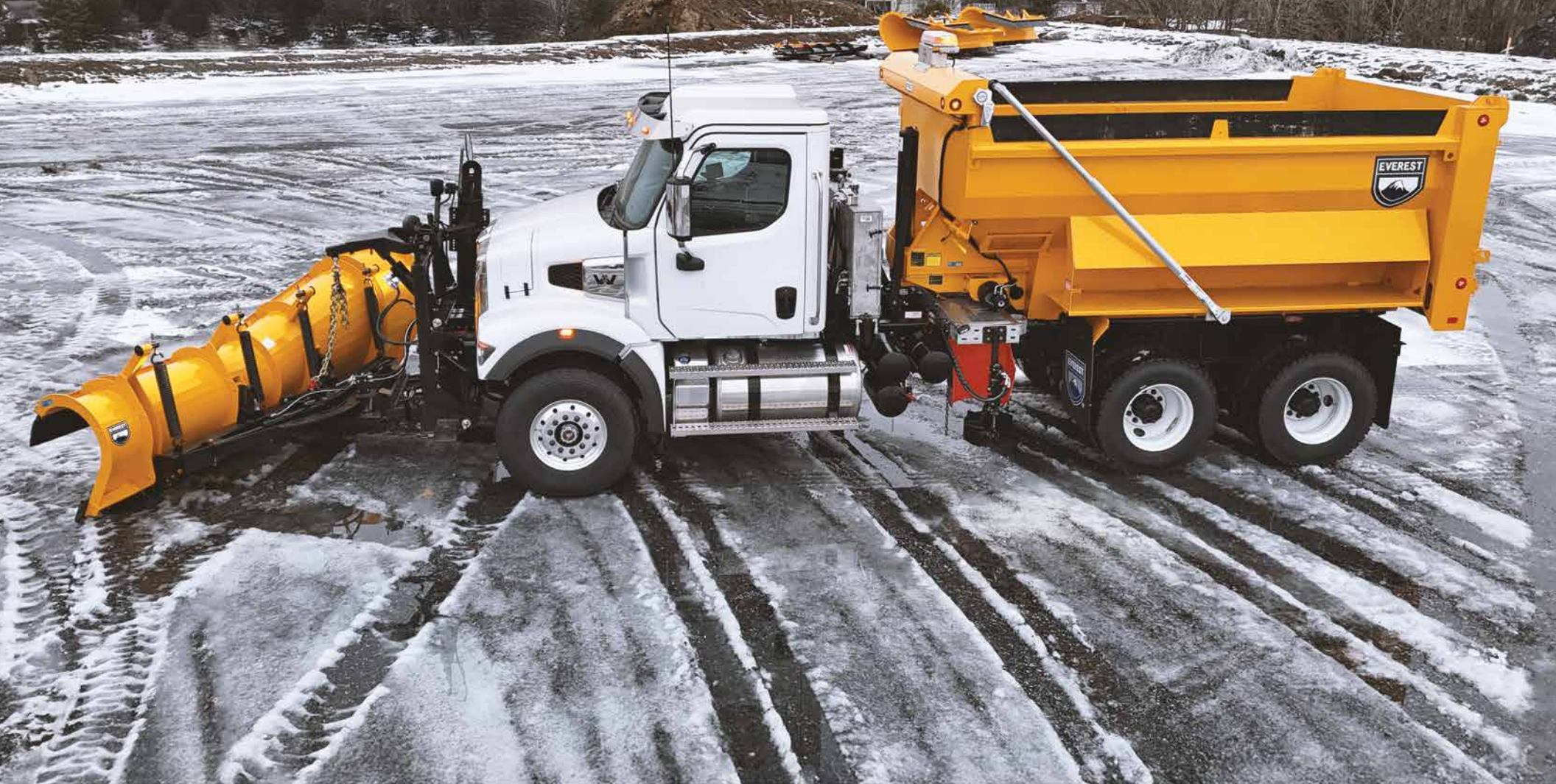
Everest heavy-duty snow removal truck with MUS four season elliptical shaped body / spreader build
