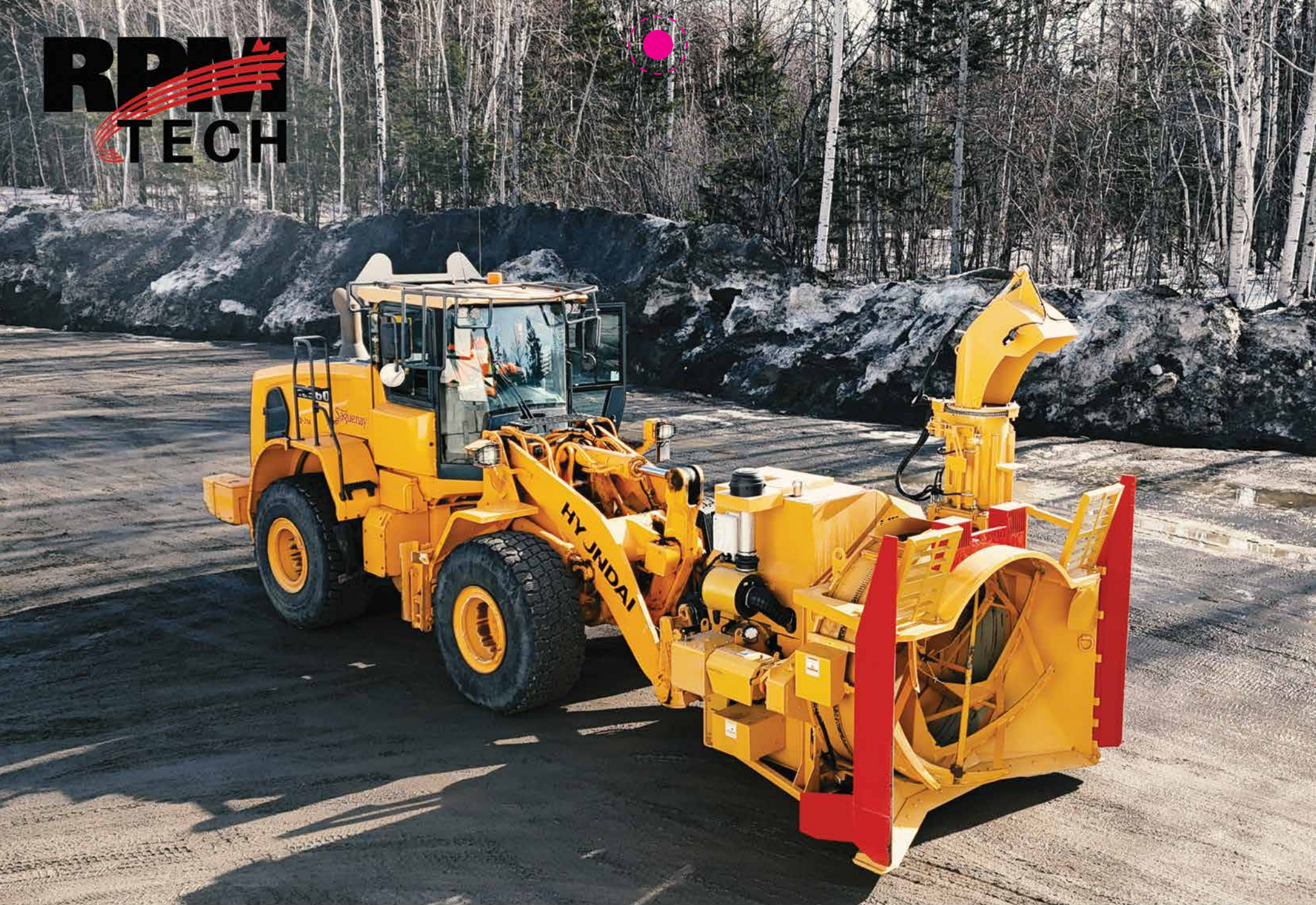
RPM Tech HS300 3,000 tons/hr single stage snow blower, ideal for snow depot or mountain passes
